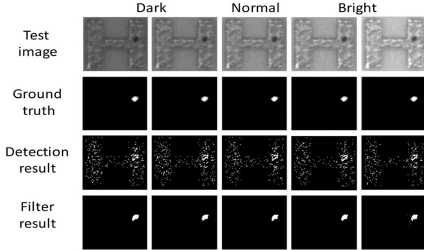
Fig.2 some example of inspection results under different illumination conditions.
